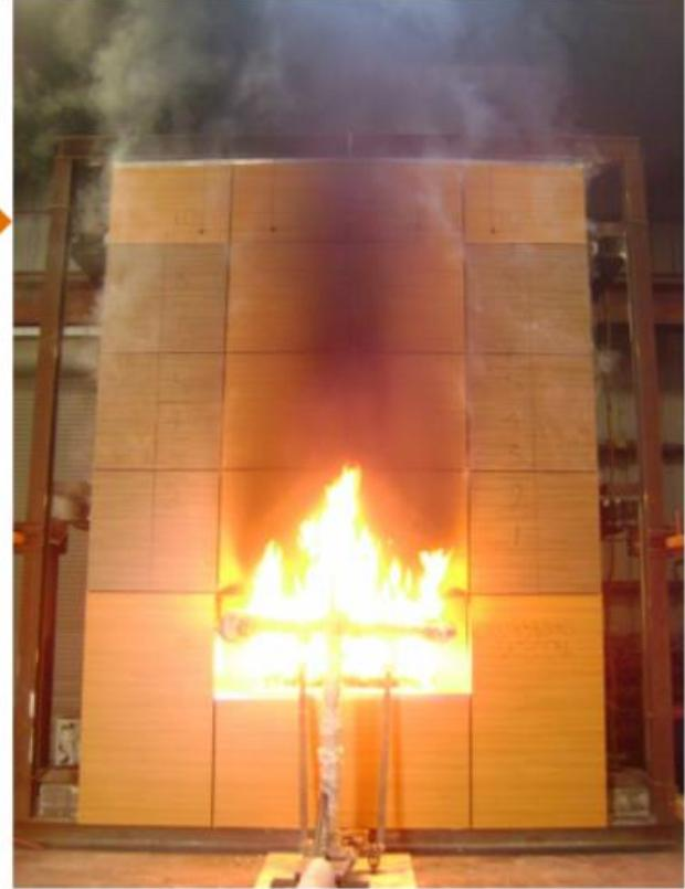
All Large-Scale Façade tests are similar in concept but very different in fire exposure conditions, test requirements, test conduct, and performance
