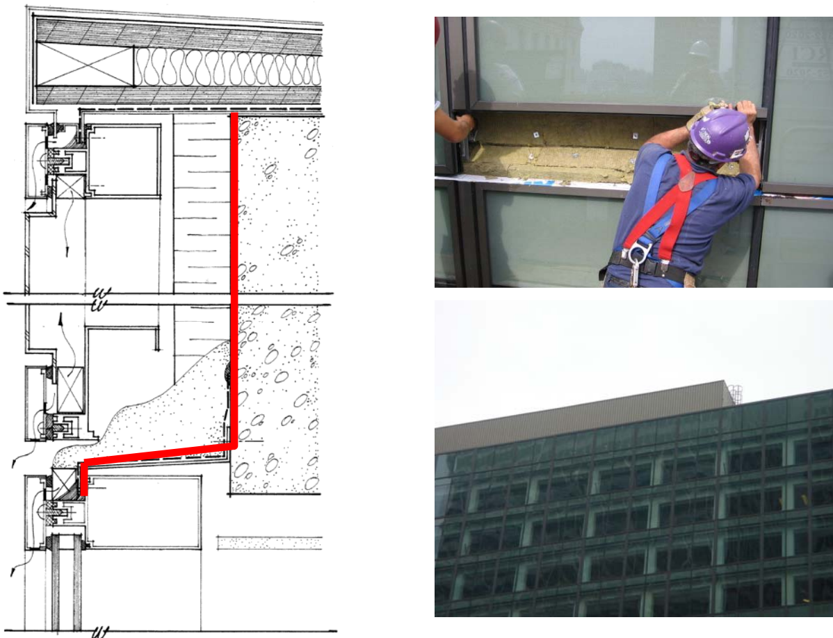
Figure 8: Curtain wall interrupted and sealed below the parapet level.
