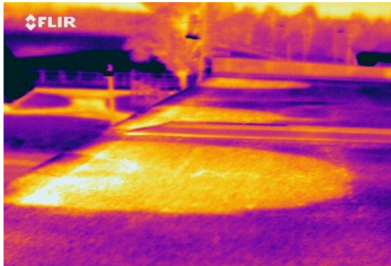
Figures 6 and 7. Typical infrared scan of wet area within roofing system at left. At right, paint typically used on roof surface to delineate suspect area of roofing system.
