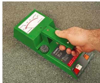
Figures 11 and 12. Use of a capacitance meter used to detect moisture in the roofing system.
